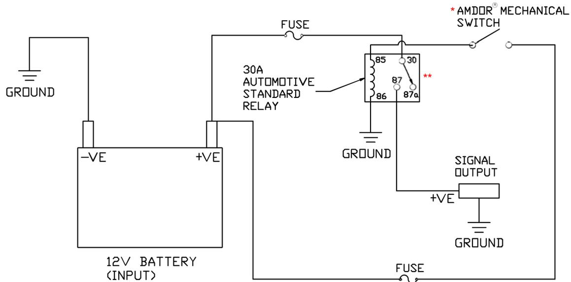
\*AMDOR MECHANICAL SWITCH RATED FOR A MAXIMUM CONTINUOUS DRAW OF 1.5A @12VDC
