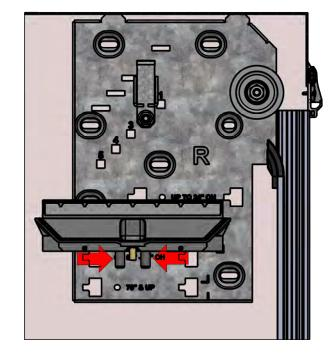
**Step 03:** Lower the DripShield until it is below the retracted latches, then release the latch handles. Support the DripShield end from the bottom while moving to the other side of the compartment and repeat step 02 on the opposite end of the DripShield in order to remove the DripShield from the compartment.
