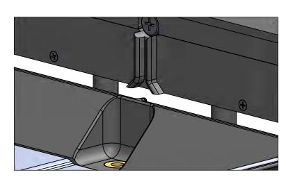
**Step 02:** Slide the DripShield up so that the angled surface on the DripShield end cap is in contact with the latches
