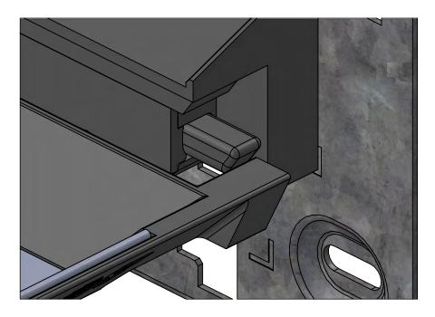
**Step 03:** Push the DripShield from the bottom past the spring loaded latches to secure in place. The latches will move out of the way of the DripShield automatically and snap back to secure the end of the DripShield in place.
