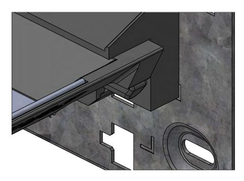
**Step 04:** Support the bottom of the DripShield while moving to the opposite side of the compartment. Repeat steps 01, 02, and 03 on the opposite side of the compartment to complete the DripShield Installation. Gently test that the DripShield is secure.
