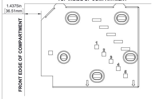
AMDOR Mounting Plate installation position from the front edge of the compartment has been changed to 1-7/16" [previously 1-5/16"]. Only the Left-Hand plate is shown here. The Right-Hand plate should be positioned at the same distance.
